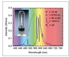
Spectrum of a high-pressure sodium lamp (solid line, OSRAM Vialox 70 W NAV(SON)-T) compared to the standard sensitivity of the human eye (dash-dotted line), with power P, luminous flux  $\Phi$ , efficiency  $\eta$ , colour temperature  $T_m$  and colour rendering  $R_a$ .
