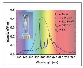
Specifications of a metal halide lamp (OSRAM Powerball HCI-T 70 W | WDL) compared to the standard sensitivity of the human eye (dash-dotted line).
